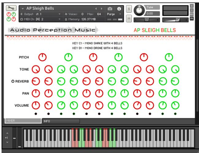
The tone control is strictly a low pass/high cut filter, to take some of the edge off the treble frequencies if needed. Turned fully clockwise is no filtering.
